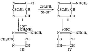
At  $50-60^{\circ}$  the product is the hydrochloride of 2-ethylmercapto-6-methylaminopyrimidine, II, while at  $150^{\circ}$  the ethylmercapto group is displaced and the hydrochloride of 2,6-di-(methylamino)-pyrimidine, III, is formed. The free bases are easily obtained from the corresponding hydrochlorides by treatment with alkali.
